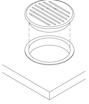
Install ZG1 into the cut out and be sure it is fully leveled onto worksurface.
