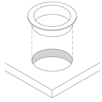
Install XG1 into the cut out and be sure it is fully leveled onto worksurface.
