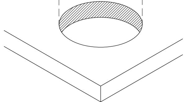
Make a cut out on the desired surface. (Note: We do not recommend cutting before receiving part or part sample.)
