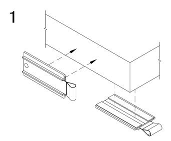
Determine the position and location on the work surface in which to apply the WM7-90NL. The WM7-90NL can be mounted underneath or on the side of the work surface.
