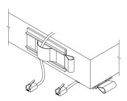
Apply pressure to the WM7-90NL until the adhesive holds the unit in position. Unstrap the Velcro fasteners so that wires may be placed in the WM7-90NL.
