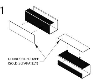
Determine whether the WM4 will be installed on the top or bottom of the work surface and apply adhesive or double-sided tape accordingly. If purchased with pre-installed double-sided tape, proceed to step 2.
