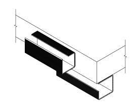
Apply pressure to the WM4 when placing against the work surface until it is held into position by the adhesive.
