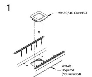
Determine orientation and push the WM39/40-CONNECT into the opening of the WM40 trough. (Note: See WM40 installation sheet for more information regarding WM40 installation.)
