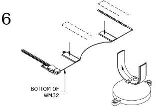
Feed the Hook and Loop straps through the WM32 weighted base. Attach the straps at the bottom of the WM32 as shown. Adjust height by changing the placements of the straps.
