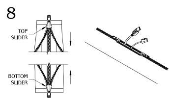
Fasten zip at each end and move sliders to desired cable exit location.
