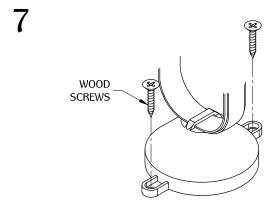
Fasten Base to floor if necessary.
