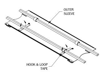
Arrange cables as desired and secure in place using
