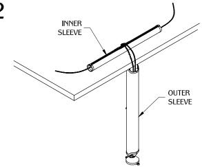
Place the Inner Sleeve of the WM32 on top of the work surface to act as a wire hub for the Outer Sleeve mounted typically.
