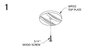
Take the WM32 Top Plate and install under the desired work surface with a 3/4" wood screw.
