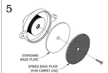
Uninstall the standard base plate and install an appropriate base plate for different floor types.
