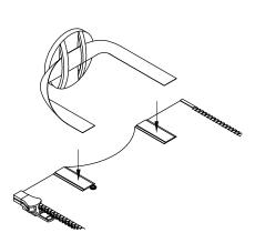
Feed the Hook and Loop straps through the top mounting plate and attach as shown. Adjust height by changing the placements of the straps.
