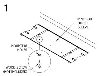
Install WM32 Inner or Outer sleeve under the desired work surface with (5) wood screws.
