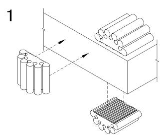
Determine the position and location on the work surface in which to apply the WM25. The WM25 can be used as a surface, under, or side mount.
