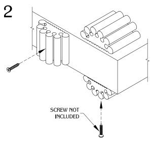
Drill a hole through the center groove of the WM25 before attaching to the work surface. Using a screw, drill through the hole that was created in the groove, attaching the unit to the work surface. Applying an adhesive to the base surface of the WM25 may be used as an alternative installation method to avoid drilling.
