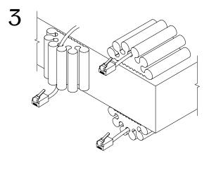
Place wires into position by slipping them through the grooves of the WM25.
