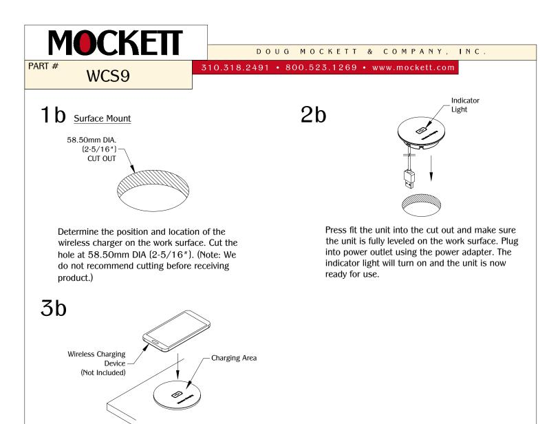
Position the mobile device on the center of the charging area. The charging icon will activate on the device's screen when properly aligned at the center of the charging area.
