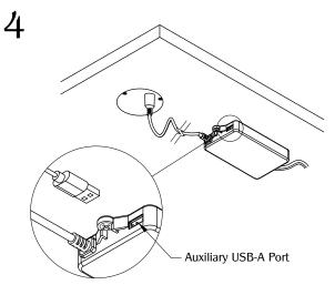
Use auxiliary USB-A port connection located on power adapter for any other powered USB connections you may need.
