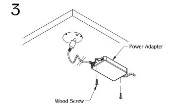
Secure power adapter under the worksurface with (2) screws. Connect adapter to the UCS1.
