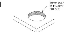
Make a cut out on the desired surface. (<u>Note</u>: We do not recommend cutting before receiving part or part sample.)
