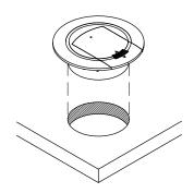
Install UCS1 into the cut out and make sure it is fully leveled onto the worksurface. UCS1 will pressure fit securely in place.
