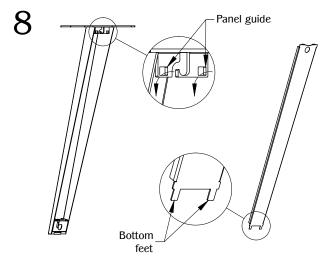
Apply the felt pad to eliminate any space between where the cover and the leg meet. Install the felt pads on top of the leg by the panel guide and the bottom feet of the cover panel.
