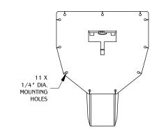
Once the orientation and table top is determined, Install the leg under the work surface. (Note: Mounting hardware is <u>not</u> included. Use the appropriate mounting hardware for the table top.)
