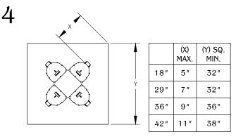
Diagonal orientation must meet requirements. (Note: Maximum table top is 60" sq.)
