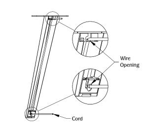
Feed the cord from the top. Hook the cord to the wire opening. Guide the cord all the way through the bottom wire opening.
