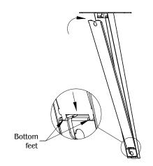
Place the cover panel by installing the feet to the bottom of the leg. Then hook the top panel cover to the panel guide. Make sure it is secure and level.
