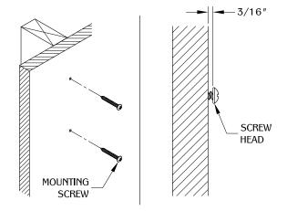
Install the (2) mounting screws. Make sure to have at least 3/16 " gap from the work surface and screw head. (Note: The gap may be adjusted to 1/8 " for a tight fit.)
