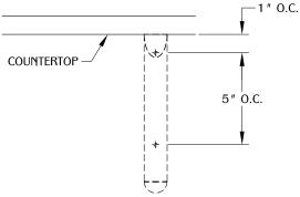
Determine the position and location of the part on the work surface. Must be installed into studs or blocking. Mark the mounting positions and drill pilot holes for the mounting hardware. Use 1 " on center from the bottom of the countertop. The part must be installed before countertop installation.
