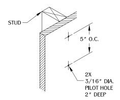
Determine the position and location of the part on the work surface. Must be installed into studs or blocking. Mark the mounting positions and drill pilot holes for the mounting hardware.
