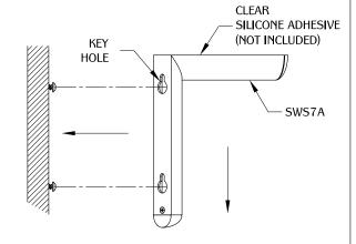
Install the SWS7A bracket by aligning the key holes to the screw head. Push down until screws are secrued in place, check if bracket is secured and adjust screw depth if necessary. For added security, we recommend a clear horizontal adhesive strip.
