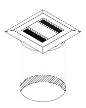
Install SQR1 into the cut out and be sure it is fully leveled onto work surface.
