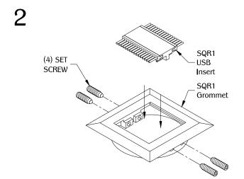
Place SQR1 insert into the SQR1 grommet. Secure using (4) set screw with a 2.5mm Allen wrench. (Note: Allen wrench NOT INCLUDED.)
