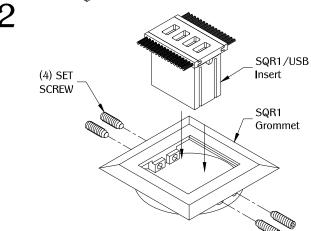
Place SQR1/USB insert into the SQR1 grommet. Secure using (4) set screw with a 2.5mm Allen wrench. (Note: Allen wrench NOT INCLUDED.)
