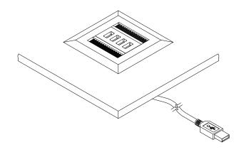
Plug-in USB cable to a USB compatible port.
