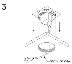
Plug-in USB cable under the SQR1/USB insert. Guide the cable into the cut out. Place SQR1/USB into the cut out and be sure it is fully leveled onto work surface.
