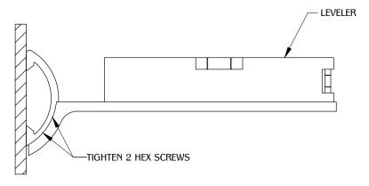
Adjust SH52 until leveled. Fully tighten screws with hex key provided.
