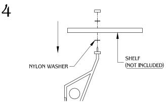
Remove the mounting cap. Use two nylon washer to protect shelf material. Align the shelf with the mounting holes and secure with mounting cap.
