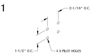
Note: Recommended to mount into wall studs.
