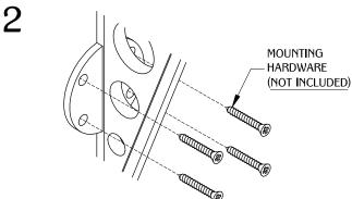
Make sure the part is leveled and aligned straight. Then, install the part with the mounting hardware(s). Repeat Step #1 for the second shelf support. (Note: Maximum bracket spacing is 30" O.C.)
