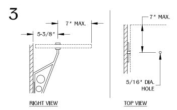
Determine the side and front over hang projection for the shelf. Then, drill the on center mounting hole on the shelf. Shelf width not to exceed 12-3/8" or a maximum of 7" overhang from the mounting post.
