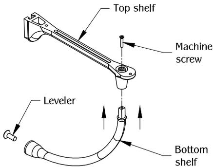
Assemble SH11 before installation by inserting the bottom shelf into the top shelf and securing with provided machine screw.
