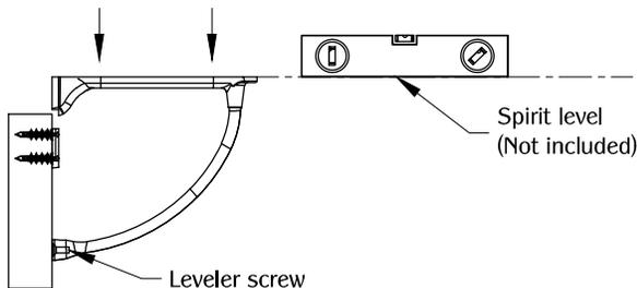
Slide down shelf support into the bracket and adjust the leveler until your shelf its leveled. (We recommend to use a spirit level not included)
