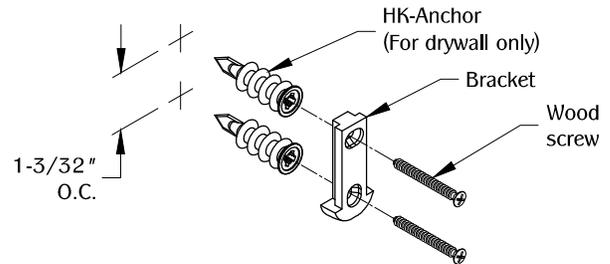
Install SH11 bracket, Make sure the its leveled and aligned straight. Then install the part with the mounting hardware provided. Repeat procedure for the second shelf support.
