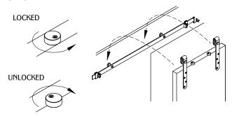
Set the door bumper to unlock. Place the assembled cabinet doors on the rail. (Note: Make sure to lock the door bumper before sliding the cabinet doors.)
