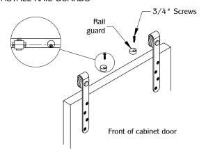
Install the rail guard on top edge of the cabinet door(s). Make sure it is aligned with the wheel of the bracket.
