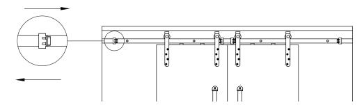
Loosen the set screws on top of the door stops by using the provided hex key. Slide the inner and outer stops to your preferred distance and setting. (Note: If the wall mount interferes with the door stop, the wall mount might need to be temporarily uninstalled.)
