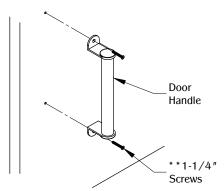
Determine the position and location of the door handle on the work surface. Secure the part by using (2) screws on each door. (Repeat 1 time) (\*\*Note: Mounting hardware not included for material thickness **less than** 1-1/4".)
