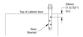
Mark the first mounting hole from the cabinet brackets. Allow 28mm (1-3/32") from the top of the door cabinet.
