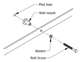
Align the Top rail to the pilot hole with the wall mount and washer. Secure the rail with the bolt screw. (Repeat 4 times)
