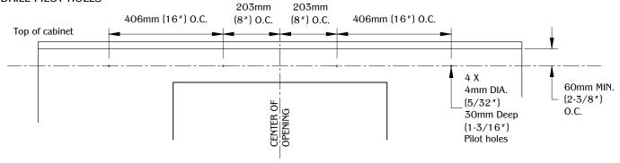
Mark the mounting positions and drill the pilot holes for the mounting hardware on the top portion of the cabinet. Make sure the pilot holes are leveled and aligned with 60 mm (2-3/8") space required.
