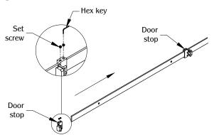
Slide a Left and Right Cabinet door stop to the <u>middle</u> of the Top Rail. Use the hex key to align and lightly tighten the set screws on top of the door stops enough for it to stay put.
