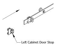
Install the outer door stop onto both ends of the top rail. Use the hex key to align and lightly tighten the set screws.
