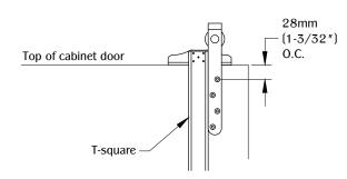
Use a T-square to line up the bracket perpendicular to the top edge. Use the 3/4" wood screws screws to secure the part. (Repeat 4 times)
