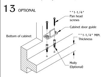
Install the door guides at the bottom of the cabinet door. (\* \* Note: Mounting hardware not included for material thickness <u>less than</u> 1-1/4".)
