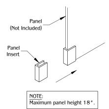
Determine the panel thickness. Attach the insert at the bottom corner of the panel. (Must use plastic inserts for 1/4" or 3/8" panel.)
