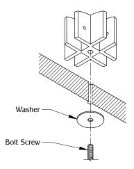
Secure the part using a 1/4 " - 20 thread screw and washer.
