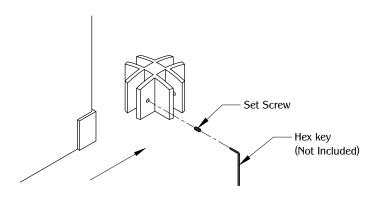
Slide the panel with the insert into the grooves of the part. Secure the panel with the set screw. (Repeat Steps #3 & #4 for other panels.)
