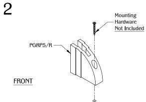
Align the PGRP5/R to the pre-drilled pilot hole. Make sure the part is fully level on the work surface. Secure the part by using a mounting hardware. (NOTE: Repeat Step #1 for the PGRP5/L and make sure both are aligned.)
