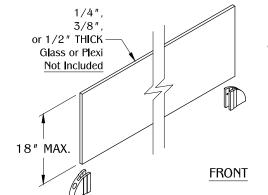
Insert your material (glass/display panel/etc) into the PGRP5 opening.
