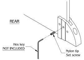
Use the hex key to secure the material with the set screw. (Note: Check tightness of screws periodically over time to ensure parts are securely tightened.)
