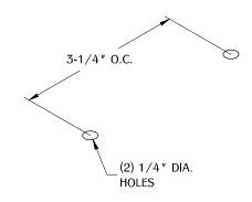
Drill two 1/4" DIA. holes at 3-1/4" O.C. in the desired work surface.
