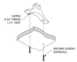
Align PGRP2 with the bottom screw holes and fasten with (2) machine screws.
