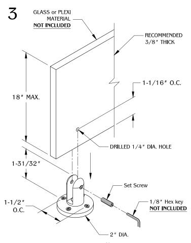
Determine where to drill a 1/4 " diameter hole at 1-1/16 " height on the material. Align pre-drilled hole with the PGRP1/B Grip. Secure the material with the (1) 3/4 " set screw.
