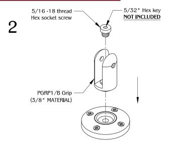
Place PGRP1/B Grip on top of PGRP1/B Base and fasten with the (1) 1/4" 5/16 - 18 thread hex socket screw.
