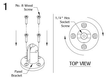
Determine the position and location of the part on the work surface. Make sure the PGRP1A is fully leveled onto the surface. Secure by using (4) No. 8 wood screws. (Note: Use a hex key to adjust panel bracket to desired orientation.)
