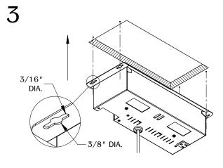
Align the unit mounting holes with the pilot holes. Secure the unit with the mounting hardware. (Mounting hardware not included.)
