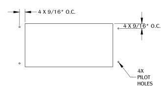
Drill (4) pilot holes to mount the unit under the work surface.
