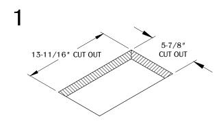
Determine the position and location of the unit on the work surface. Cut the hole at 13-11/16" X 5-7/8" from the top.
