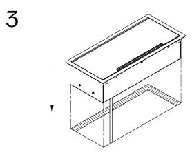
Install the unit into the cut out and be sure it is fully level on the surface.
