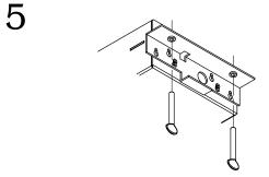
Tighten the (2) thumb screws on the mounting bracket. Plug the unit into nearby outlet (outlet should be close enough to where power cord is not taut or strained) and unit is ready for use.
