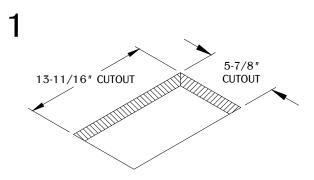
Determine the position and location of the unit on the work surface. Cut the hole at 13-11/16" X 5-7/8" from the top.
