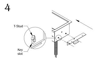
Align the mounting bracket key slots to the T-studs under the unit.
