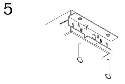
Tighten the (4) thumb screws on the mounting bracket. Connect the hardwires (Hardwire connection <u>MUST</u> comply with local electrical code.) and unit is ready for use.
