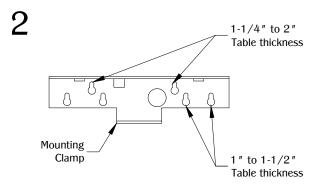
Determine the table thickness. Use the recommended guide above for the key slots on the mounting bracket.
