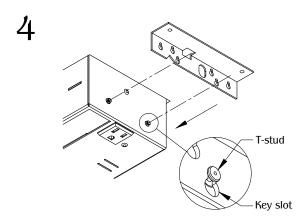
Align the (2) mounting bracket to the desired key slots to the T-studs on both sides under the unit.
