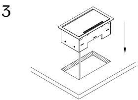
Guide the power cord through the cut out. Install the unit into the cut out and make sure it is fully leveled onto the surface.
