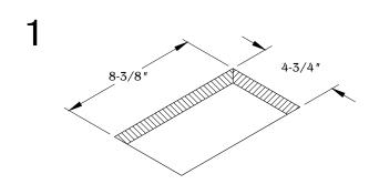
Determine the position and location of the unit on the work surface. Make a 8-3/8" X 4-3/4" cut out. Place and allow enough clearance for unit operation. DO NOT place unit where cable is strained or trapped.
