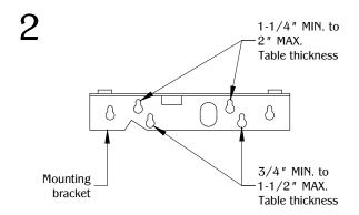
Determine the table thickness of the work surface. Use the appropriate key slots on the mounting bracket.
