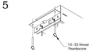
Install and tighten the (2) 10 -32 thread thumbscrews on the mounting bracket on both sides until unit is secure. Plug the unit into nearby outlet and unit is ready for use.
