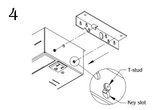
Align the (2) mounting bracket to the desired key slots to the T-studs on both sides under the unit.
