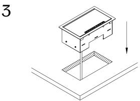
Guide the power cord through the cut out. Install the unit into the cut out and make sure it is fully leveled onto the surface.
