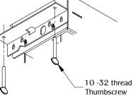
Install and tighten the (2) 10- 32 thread thumbscrews on the mounting bracket on both sides until unit is secure. Plug the unit into nearby outlet and unit is ready for use.
