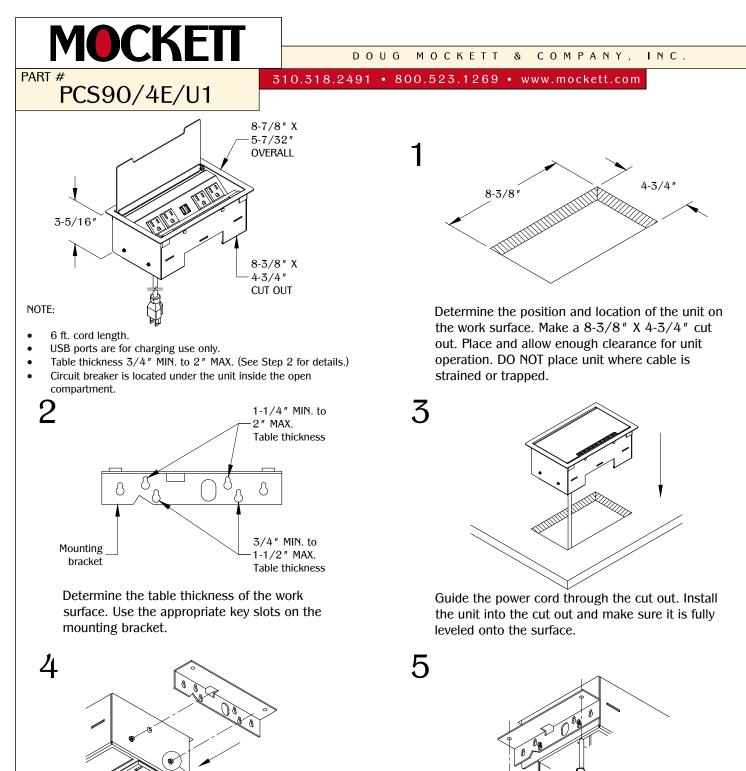
Key slot Align the (2) mounting bracket to the desired key slots to the T-studs on both sides under the unit.
