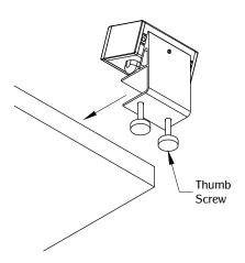
Loosen the (2) thumb screws to install the unit at the desired edge of the work surface.
