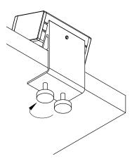
Make sure the unit is fully leveled the on the work surface. Secure the unit by tightening thumb screws. Plug the unit into nearby outlet (outlet should be close enough to where power cord is not taut or strained) and unit is ready for use.
