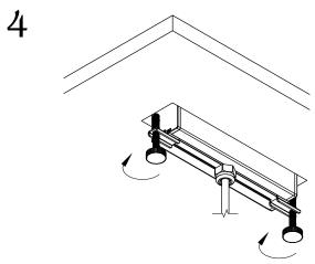
Hand-tighten the thumb screws until the unit is secure. Plug the unit into nearby outlet and unit is ready for use.
