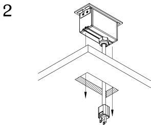
Guide the cord through the cut out. Install the unit into the cutout and make sure it is fully level on the surface.
