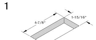
Make a cutout in the desired location on your work surface. Allow enough clearance for unit operation. DO NOT place unit where the cable is strained or trapped.
