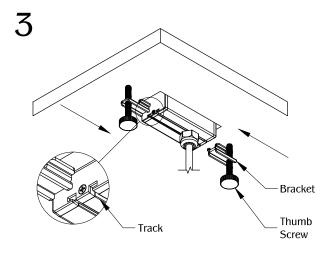
Slide the (2) mounting bracket on to the track at the bottom of the unit. Secure the part by using the (2) thumb screws.
