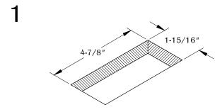
Make a cutout in the desired location on your work surface. Allow enough clearance for unit operation. DO NOT place unit where the cable is strained or trapped.
