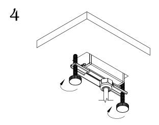
Hand-tighten the thumb screws until the unit is secure. Plug the unit into nearby outlet and unit is ready for use.
