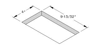
Make a cut out in the desired location on your work surface. Place near a power outlet and allow enough clearance for unit operation.  $\underline{DO\ NOT}$  place unit where the cable is strained or trapped. Cut a hole at  $9-13/32"\ X\ 4"$ .
