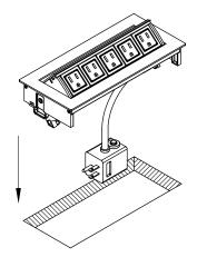
Guide the power cord through the cut out. Install the unit into the cut out and make sure it is fully leveled onto the surface.
