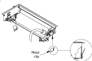
Place metal clips in the slots on the side of the unit. (NOTE: Metal clips are for use in hard surface material only as an optional mounting means.)
