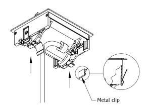
Place metal clips in the slots on the side of the unit. (NOTE: Metal clips are for use in hard surface material only as an optional mounting means.)
