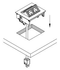
Guide the power cord through the cut out. Install the unit into the cut out and make sure it is fully leveled onto the surface.
