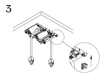
Use (4) wing clamps to secure the unit.
