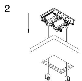
Guide the cord into the cut out. Make sure the unit is fully leveled on the work surface.
