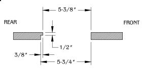
Determine which way the unit is facing. Rout out an additional 3/8" wide from the back of the cut out, providing a 15-1/4" x 5-3/4" recess. Leave 1/2" depth from the top at the rear of the cut out.
