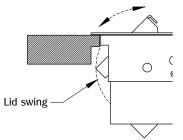
Make sure the lid operates smoothly in the cut out. Make additional adjustments if necessary. Plug the unit into nearby outlet (outlet should be close enough to where power cord is not taut or strained) and unit is ready for use.
