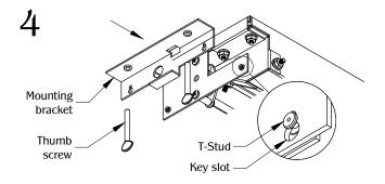
Align the mounting bracket key slots to the T-studs under the unit. Use the thumb screw to tighten and secure in place.
