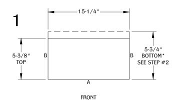
Determine the position and location of the unit on the work surface. Cut the hole at 15-1/4 " X 5-3/8 " from the top.
