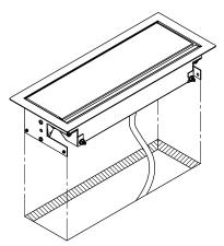
Install the unit into the cut out and be sure it is fully level on the surface.
