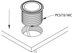
Remove the lock ring from the unit. Guide the cord through the cut out and install the unit. Make sure it is fully level on the surface.
