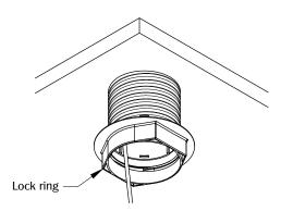
Guide the cord through the lock ring and secure the unit by tightening clockwise.
