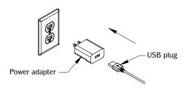
Plug in the USB plug from the unit to the power adapter. Plug the unit into nearby outlet (outlet should be close enough to where power cord is not taut or strained) and unit is ready for use.
