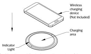
Position the mobile device on the center of the charging area. The indicator light activates to signify that the device is actively charging or the charging icon will activate on the device's screen.
