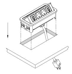
Guide the power cord through the cut out. Install PCS68/2E/U2 into the cut out and make sure it is fully leveled onto surface.
