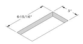
Make a cut out in the desired work surface. (NOTE: Table thickness must be at least 3/8 " minimum.)
