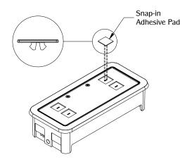
Align the Snap-in Adhesive pads to the top of the unit.
