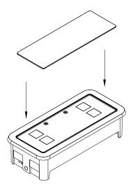
Peel off the adhesive backing on four places.
