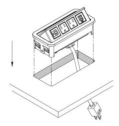
Guide the power cord through the cutout. Install PCS68/2EU1 into the cutout and make sure it is fully leveled onto surface.
