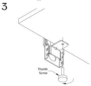
Secure the unit by aligning the thumb screw to the bracket and turning clockwise.
