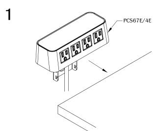
Install the unit at the desired edge of the work surface. Make sure the unit is fully leveled onto the work surface. Do NOT place unit where cable is strained or trapped.
