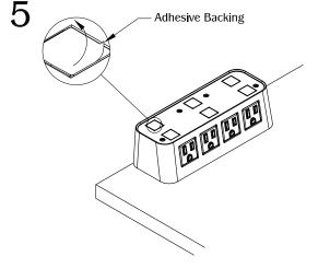
Peel off the adhesive backing on all six snap-in adhesive pads.
