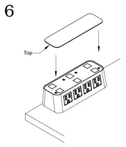
Align the top to the unit. Make sure it is fully leveled onto the top surface. Plug the unit into a nearby outlet and unit is ready for use.
