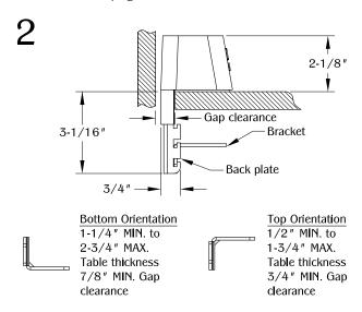
Determine the table thickness and orientation of the bracket. Install the bracket to the back plate of the unit.
