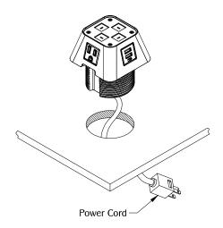
Guide the power cord through the cut out. Install PCS66G/2/U2 into the cut out and make sure it is fully leveled onto surface.
