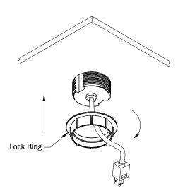
Guide the power cord through the lock ring. Secure the unit by turning the lock ring clockwise.
