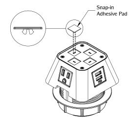
Align the Snap-in Adhesive pads to the top of the unit.
