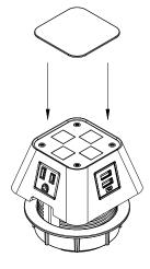
Peel off the adhesive backing on 4 places.
