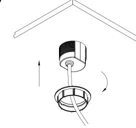
Remove the Lock ring. Guide the power cord through the cut out. Install PCS65/USB into the cut out and make sure it is fully leveled onto surface.
