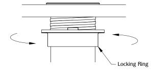
Guide the cord through the cut out. Install the unit into the cutout, make sure it is fully level on the surface, and oriented to the appropriate side.
