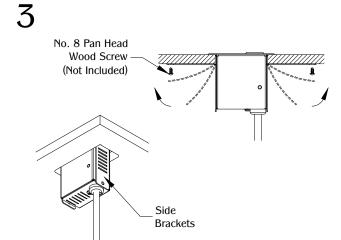
Bend the (2) side brackets and use (2) pan head wood screws to secure unit under the work surface.
