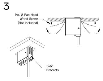
Bend the (2) side brackets and use (2) pan head wood screws to secure unit under the work surface.
