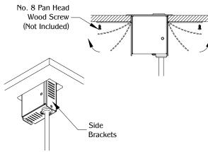
Bend the (2) side brackets and use (2) pan head wood screws to secure unit under the work surface.
