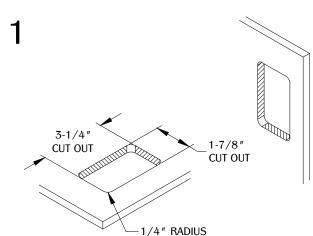
Determine the position and location of the unit on the work surface. Cut the hole at 3-1/4 " X 1-7/8". Place and allow unit operation. Do not place unit where the cable is strained or trapped.
