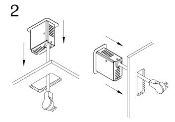
Guide the power cord through the cut out. Install the unit into the cut out and make sure it is fully leveled on the work surface.
