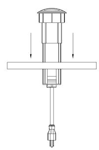
Install the PCS6/EE/M into the cut out and be leveled onto the work surface.
