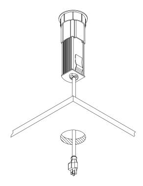
Guide the power cord through the cut out.
