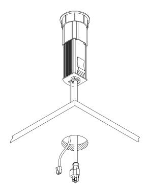
Guide the power cord and patch cord through the cut out.
