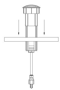
Install the PCS6/DE/M into the cut out and be leveled onto the work surface.
