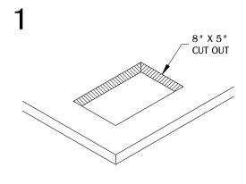
Make a cut out in the desired location on your work surface. Allow enough clearance for unit operation. DO NOT place unit where cable is strained or trapped.
