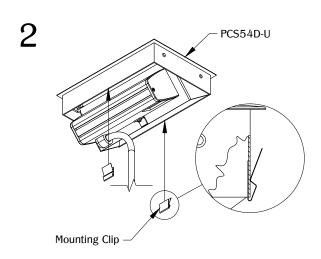
Attach the mounting clips to the front and back side of the frame on the PCS54D.
