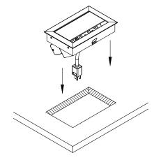
Install the PCS54D into the cut out and make sure it is fully leveled onto the work surface. Plug into a nearby outlet and unit is ready for use.
